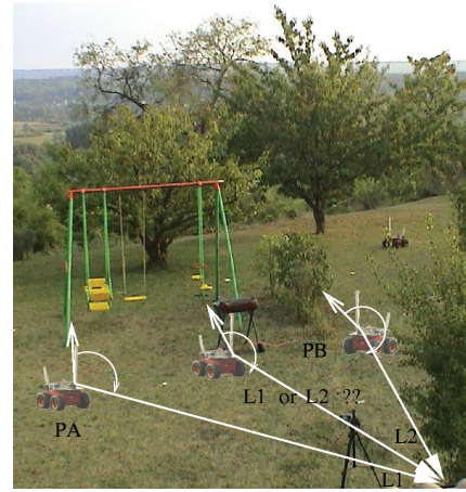
Fig. 6: Learning using the same physical landmark seen from two different points of view. The same focus point is the center of L_1 in P_A , and L_2 in P_B . During navigation, two interpretations of the same physical landmark can compete and bias place recognition.
