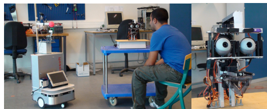
Figure 1: Experimental set-up : a robotic head that learns facial expression recognition and a mobile robot able of autonomous visual navigation tasks learning. The room size is 7m x 7m, but the robot's movements are restricted to an area of 3m x 3m (to allow a good video tracking of the robot's trajectories).
