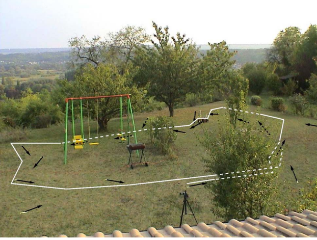
Fig. 6. Outdoor environment and looped sensory-motor trajectory. The arrows represent the learned positions and the associated movements. The robot closes the loop of about 100 m in 20 min. The system is slow because the entire architecture was executed by a single sequential program (September 2005).
